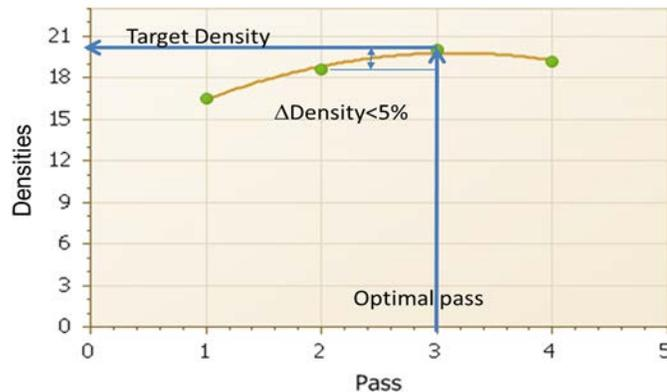
Linear regression relationships between the point test results and the IC-MV results will be used to establish the production target IC-MV as the target density (%  $G_{mm}$ ) meets the *xxDOT* in-place compaction requirements. The target ICMV is recommended only for QC. A linear regression curve example is as follows.
